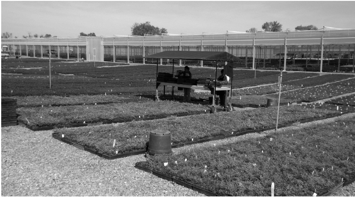
Figure 5. A typical workstation that is uncomfortable, inefficient, difficult to manage, and can lead to injury (due to the repeated bending required).
