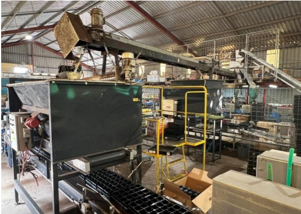
Figure 2. Soil mixing systems developed and offered by KW Automation.
