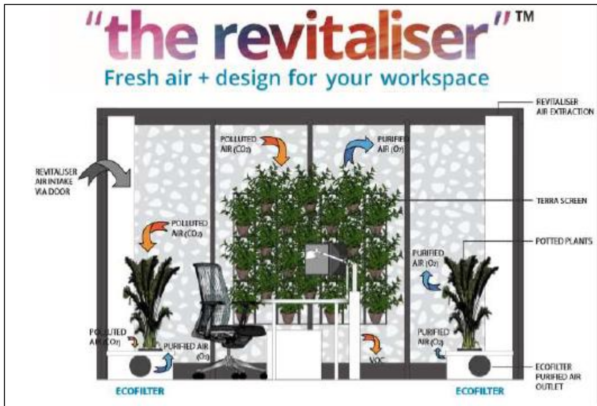
Figure 9. Conceptual diagram of Revitaliser by Eco Effective Solutions.
