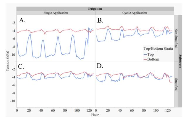
**Figure 3.** Substrate water potentials calculated via elbow tensiometers in the upper and lower portions of the container under single or cyclic irrigation application scheduling over 6 d. Treatments include A) Non-stratified substrates within a single application irrigation B) Non-stratified substrates within a cyclic irrigation application C) Stratified substrates in a single application and D) Stratified substrates within a cyclic irrigation application.
