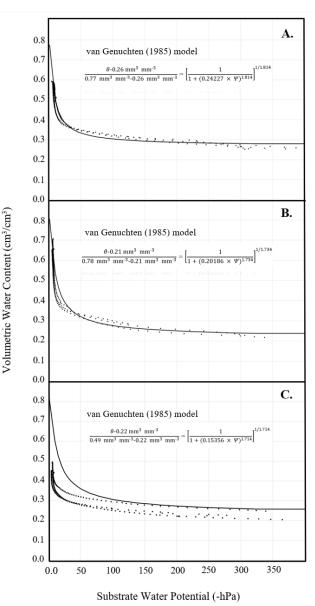
**Figure 2.** Substrate moisture characteristic data (points) fit to a constrained van Genuchten (1985) hydraulic model (solid line). The data was measured via evaporative measurement and porometers on three replicates of each substrate. Substrates include A) conventional bark, B) fine bark (<6.3 mm) and C) coarse bark (>6.3 mm). Volumetric water content (cm<sup>3</sup> cm<sup>-3</sup>; Y-axis) was plotted against substrate water potential (-hPa; X-axis).
