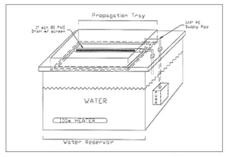
Figure 1. Three dimensional design of a recirculating subirrigation unit.
