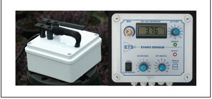
Figure 1. The Evaposensor (left) and the Evaposensor Control Interface (right).
