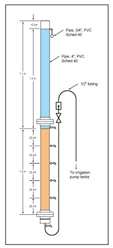
Figure 2. Sand filters for experimentation were constructed of 4-ft PVC pipe and included valves that enabled collecting samples above the sand bed, at 20-cm intervals down the sand bed, and below the bed.
