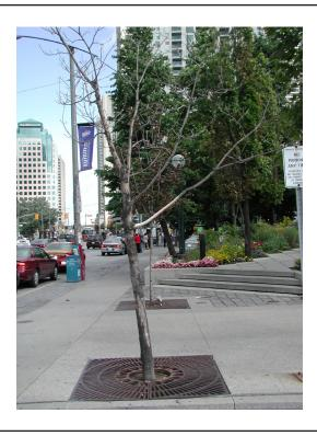
**Figure 2.** The dead tree in the foreground survived 5 years with minimal contribution to the city green space, while the group of trees in the background in a  $12 \times 18$  m ( $40 \times 60$  ft) elevated bed had sufficient space for root growth, allowing the trees to function for a number of years.
