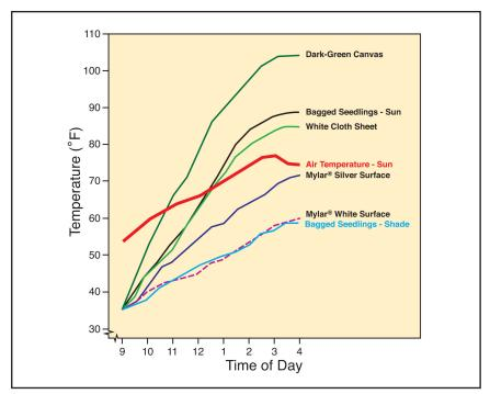
Figure 6. Research has shown that reflective Mylar<sup>®</sup> tarps provide much better insulation than standard green canvas ones (modified from (DeYoe et al., 1986).
