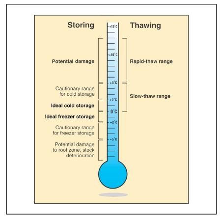
**Figure 4.** The actual temperature difference between cooler and freezer storage is minimal but those few degrees cooler make a tremendous difference in storage duration. Warmer temperatures are recommended for thawing frozen stock.
