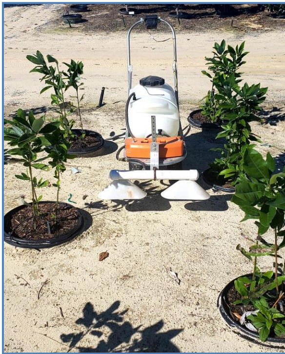
Figure 1. Jacto PJB16 battery powered backpack. Used for watering in granular herbicide applied to pot-n-pot containers.
