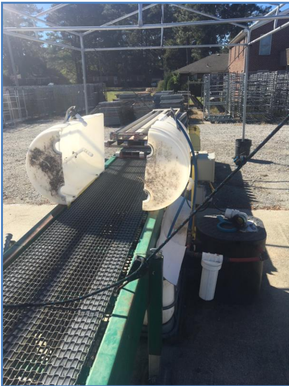
Figure 4. To make sure container walls are clean and free of dirt, the spray system in the shipping area was built which cleans the container as they move along the conveyor belt system during the loading of trucks.
