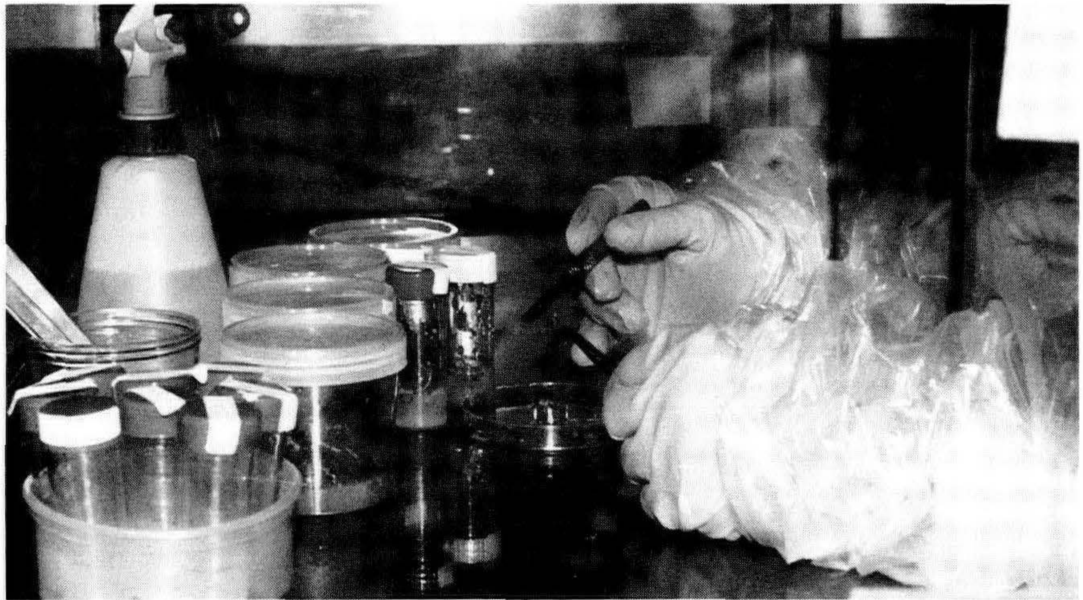
Figure 1. A transfer chamber made from a modified aquarium.
