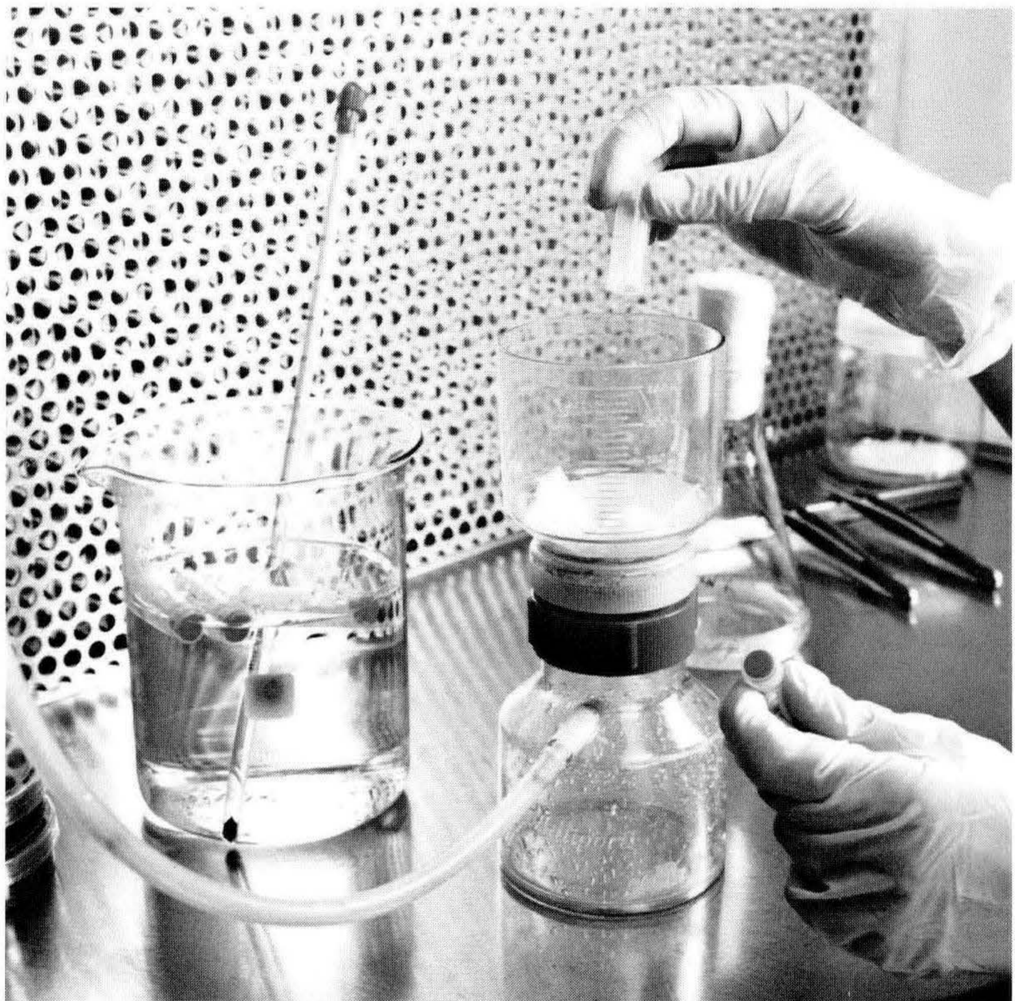
Figure 1. Thawed samples are poured onto a nylon screen in a millipore filter unit.
