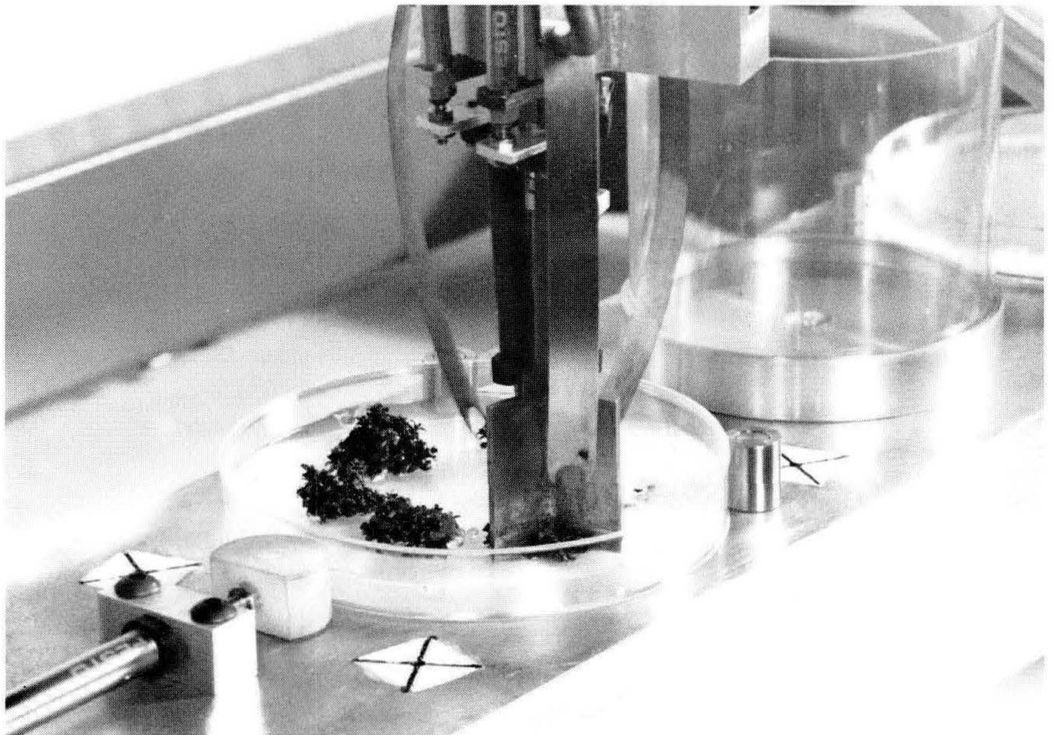
Figure 2. Robotic hand shown here cutting Eucalyptus camaldulensis .
